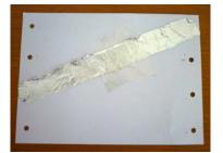
Add the next foil strip to join a different pair of holes. Make sure it does not touch the foil from the other strip! Add more sticky tape if necessary.
