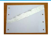
Cover the central part of the foil with stick tape. This will prevent electricity flowing between this foil strip and the next one.
